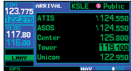
Selecting a frequency on the NAVCOM page.
